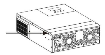
Step 6: Turn on the solar storage inverter
