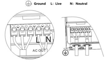
**Note:** The grounding wire shall be as thick as possible (cross-sectional area is not less than 4mm<sup>2</sup>). The grounding point shall be as close as possible to the solar storage inverter. The
